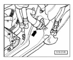
· Remove coolant hose (release clamp -arrow-).
