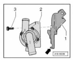
NEW auxiliary coolant pump, installing:
