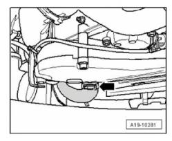
• Disconnect coolant hose -arrow- from thermostat housing port.
