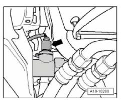
• Disconnect electrical connector from thermo switch on lower end of coolant hose to radiator -arrow- .
