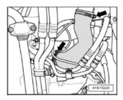
• Remove lower pressure hose to charge air cooler (right side).
