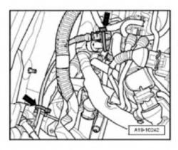
Secure connected harness with 2 Tie Wraps -arrows- as shown.
