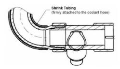
• Install shrink tubing (Part No: 078 121 092) onto coolant hose as shown in cross section.
