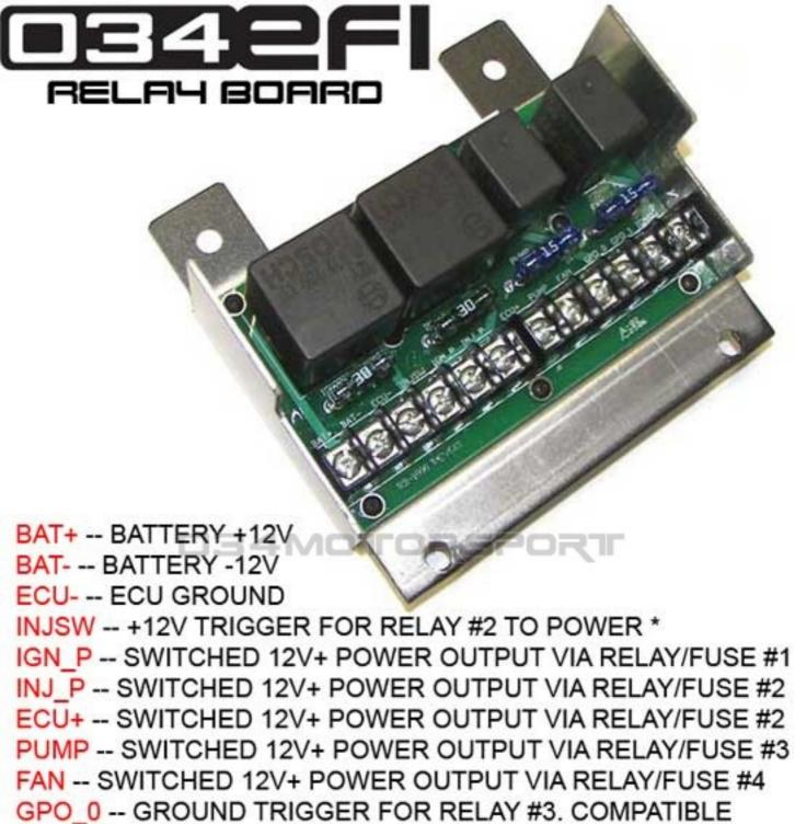
WITH ALL GPO OUTPUTS ON 034EFI ECU'S GPO 1 -- GROUND TRIGGER FOR RELAY #4. COMPATIBLE WITH ALL GPO OUTPUTS ON 034EFI ECU'S IGNSW -- +12V TRIGGER FOR RELAY #1 \*
