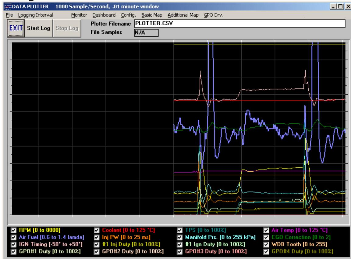
The Plotter is a useful datalogging feature of the 034EFI “C” ECU’s, it allows ECU data to be recorded and saved to the laptop hard drive for future analysis. This is especially useful as there is typically a large amount of hard-drive space available for extended, almost unlimited amounts of datalogging time.
