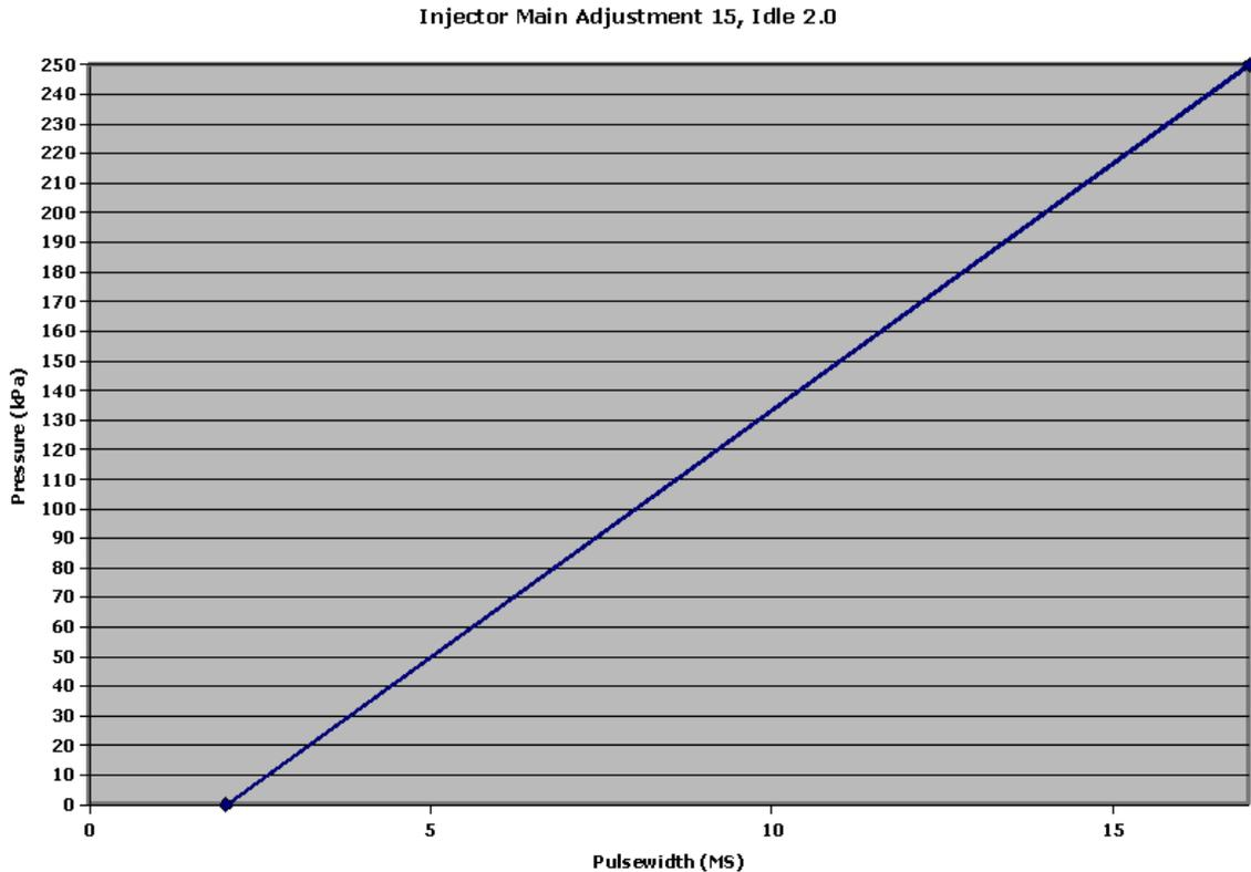
Injector Main Adjustment 15, Idle 0.0
