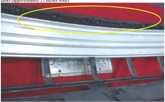
Remove material to clear end tanks on the left and right sides of the bumper cover.
