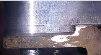
Step 2: Install the provided socket-head bolt thru the Apikol Sway bar bracket and the shock mount casting. Rotate the Apikol bracket downward to engage the locking tank against the shock mount. Center-punch for the M8x1.25 screw in this position, then drill/tap the casting.
